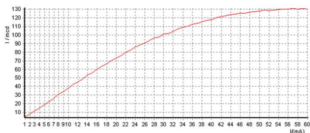
电流-光强曲线 Current-Luminous intensity Curve
